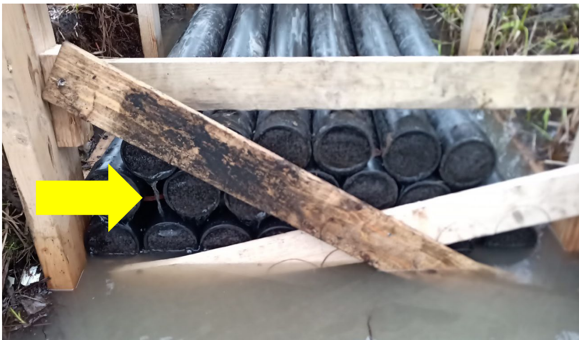
Fig. 18. Pipe filter prototype. View of the downstream sections. Part of the flow passes through the voids between the pipes while the rest passes through the pipes filled with filter granulates. The yellow arrow shows water dripping from a pipe above the downstream water level, indicating a higher water level on the upstream side.
