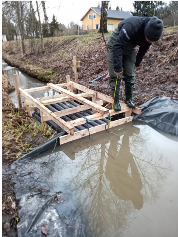
Fig. 19. The pipe filter design during the testing phase. The tarpaulin in the upstream section was added to minimize erosion during higher discharge conditions.
