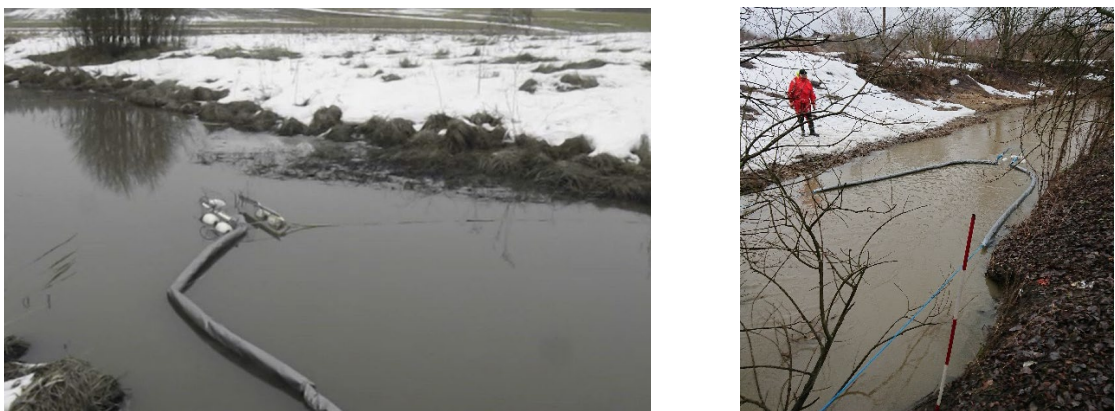
Fig. 12. Litter trap testing during high water level but low flow velocities in left) Jaaninoja and right) Kuninkoja, March 2019.
